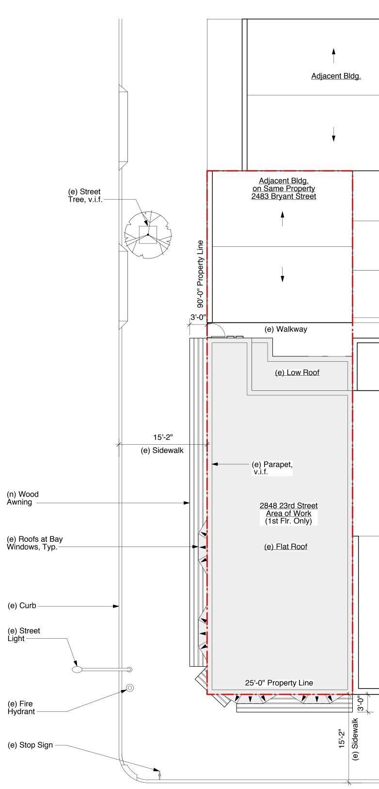
2 Proposed Site Plan Scale: 1/8" = 1'-0"
