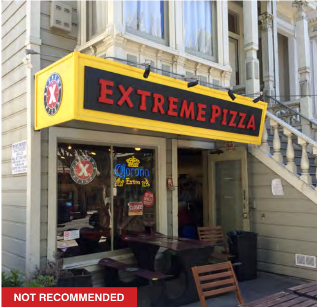
Scale of sign is inappropriate and extends beyond the storefront entrance.
