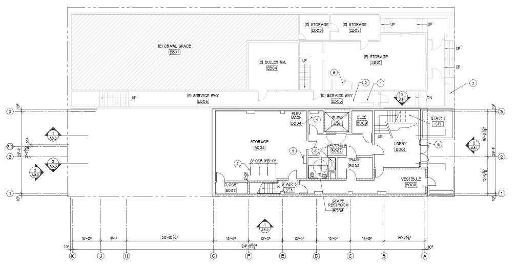
BASEMENT FLOOR PLAN — SCALE : 1/8" = 1'−0'
