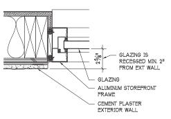
$3 \ \, \underset{\text{SCALE : } 3"=1'-0"}{\text{TYPICAL WINDOW JAMB}}$
