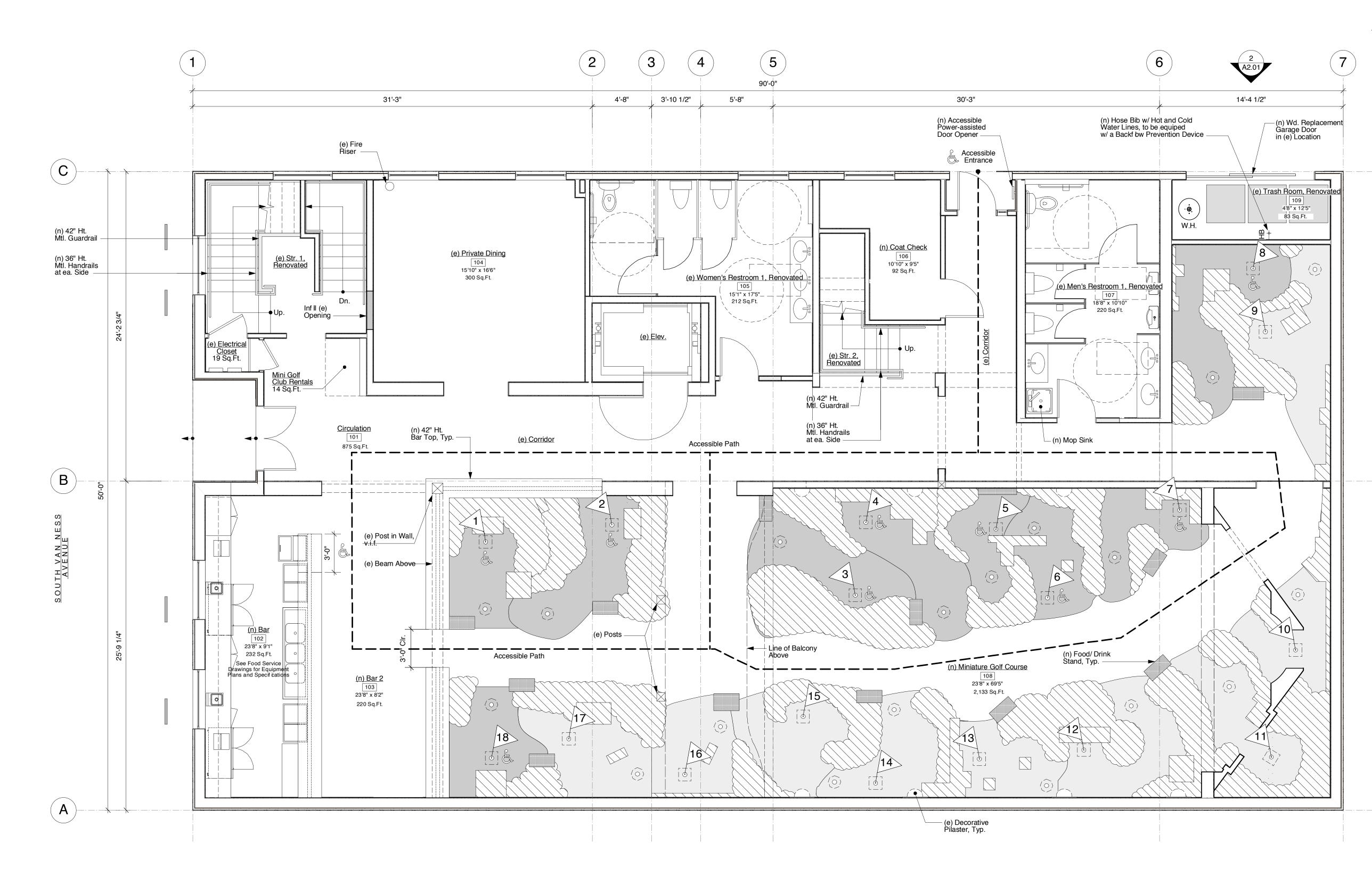
1 Proposed First Floor Plans Scale: 1/4" = 1'-0"
