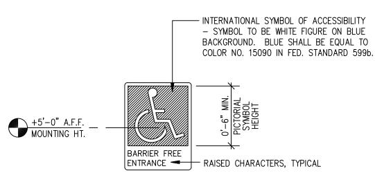
NOTE: "SIGNS SHALL BE INSTALLED ON THE WALL ADJACENT TO THE LATCH OUTSIDE THE DOOR. WHERE THERE IS NO WALL SPACE ON THE LATCH SIDE, INCLUDING AT DOUBLE LEAF DOORS, SIGNS SHALL BE PLACED ON THE NEAREST ADJACENT WALL, PREFERABLY ON THE RIGHT. MOUNTING SHALL BE DETERMINED SO THAT A PERSON MAY APPROACH WITHIN 3 INCHES OF SIGNAGE WITHOUT ENCOUNTERING PROTRUDING OBJECTS OR STANDING WITHIN THE SWING OF THE DOOR."
