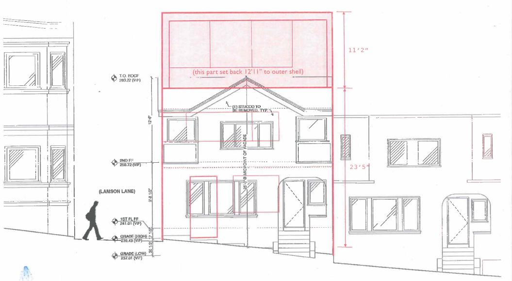
Front view from 19th Street of proposed structure (red) superimposed upon existing structure (black). All objects are drawn exactly to scale from plans provided. Walking man is 5'10".
