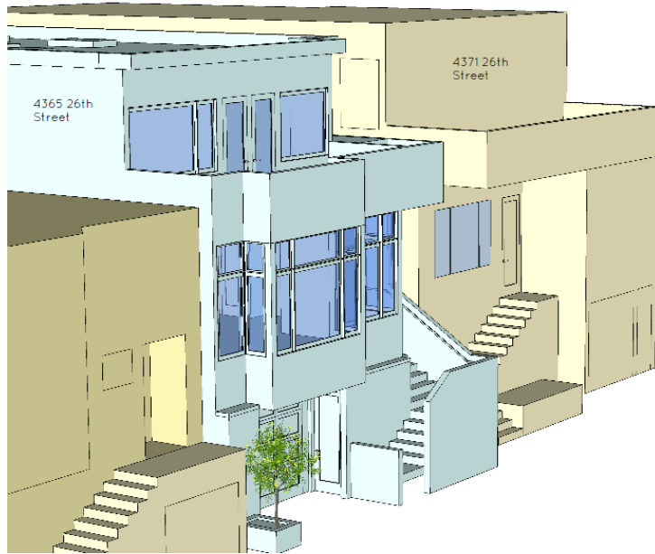
3D shows no protrusions in front of 4371. Also visible is saved lot-line window.
