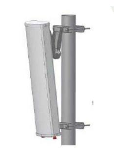
Features at a Glance: • 90° x 30° sector • 10 dBi peak gain at 2.4 and 5 GHz • 2400-2483.5 and 4900-5900 MHz Four N-female connectors • Linear dual slant 45° 2x2 at 2.4 / 5 GHz
