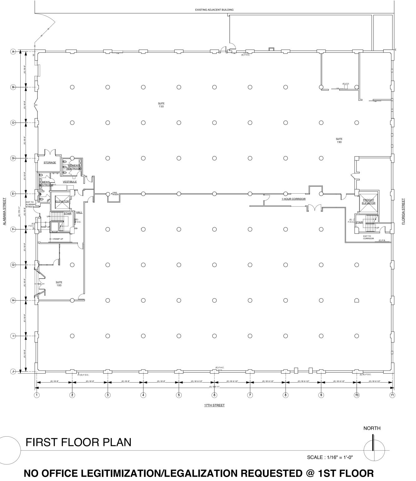
**1ST FLOOR AREA LEGEND** (GROSS FLOOR AREA MEASURED PER S.F.PLANNING CODE SEC. 102.9) TOTAL GROSS FLOOR AREA = APROX. 37,297 SF
