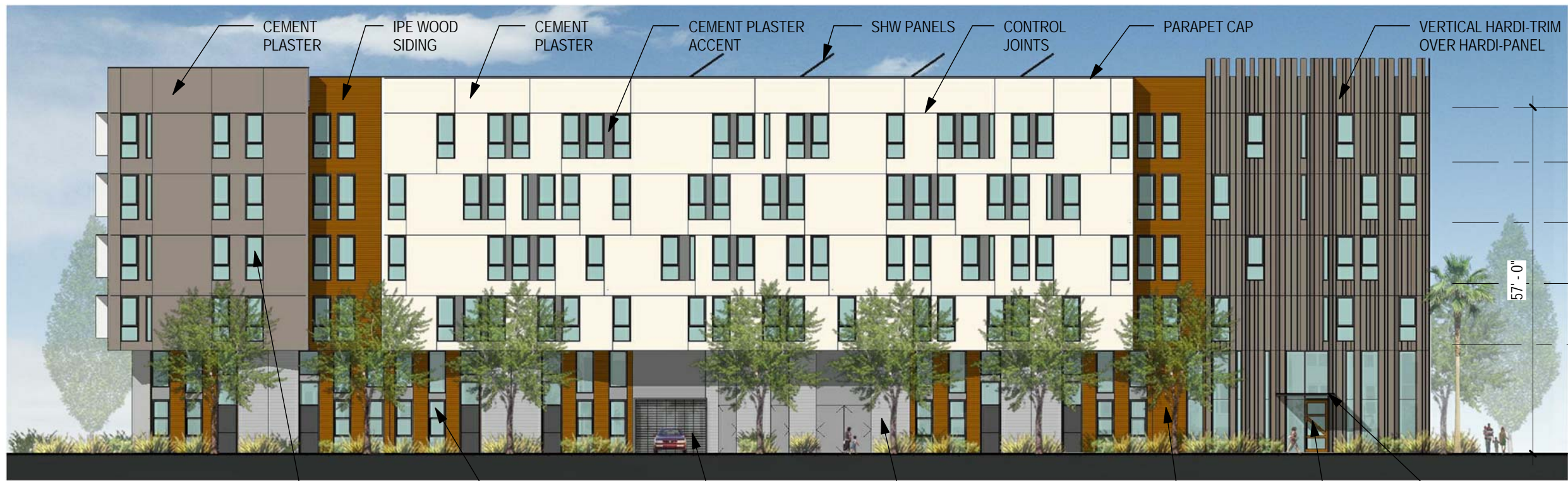
② EAST ELEVATION - PRIVATE ROAD (LOT 41) 1" = 20'-0" Labels: FIRE ACCESS EASEMENT, THERMALLY BROKEN ALUMINUM WINDOWS, STOREFRONT WINDOWS, GARAGE, BOARD FORM CONCRETE, IPE WOOD SIDING, WOOD ENTRY DOOR, STEEL AWNING, SOUTH MEWS.
