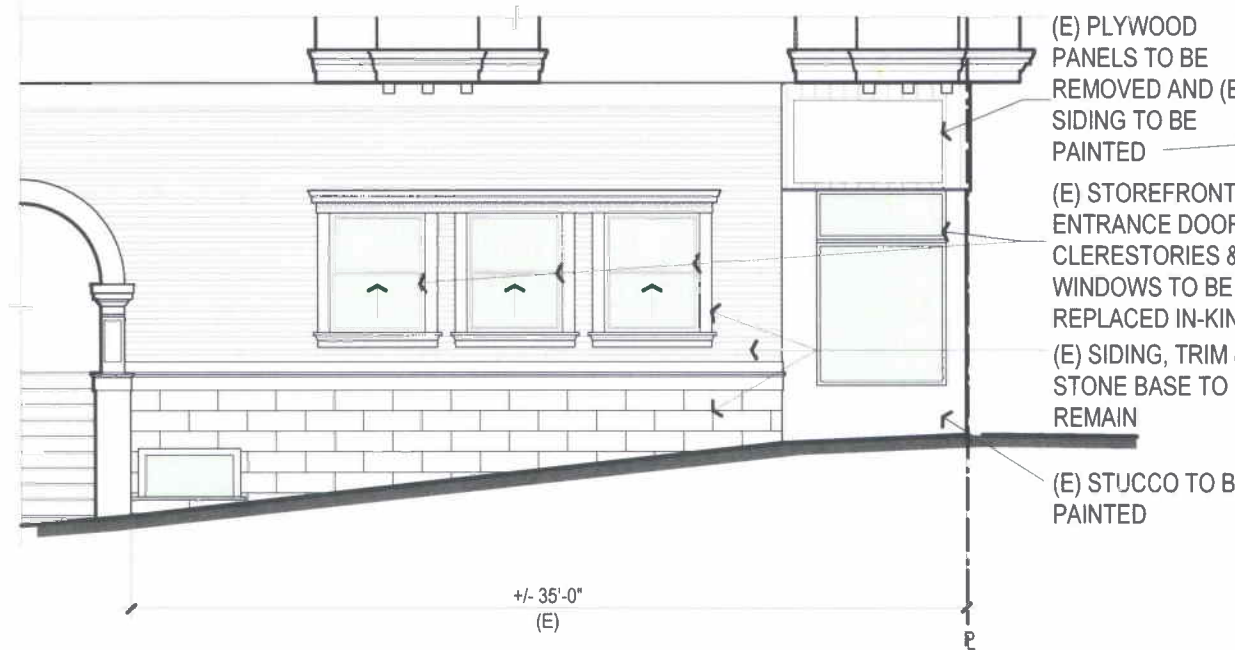
EXISTING EAST ELEVATION
