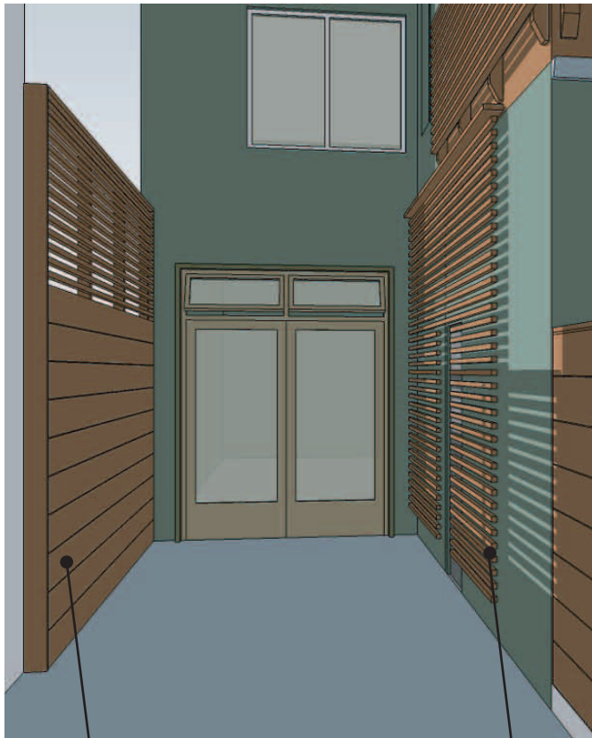
New wood slats/planting on existing wall to dissipate sound at the proposed seating area
