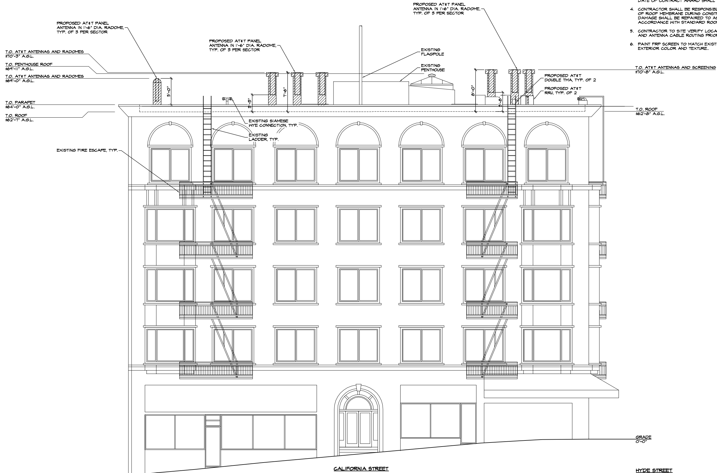
CALIFORNIA STREET SOUTH ELEVATION 3/32"=1'-0" 0 2' 4' 8'
