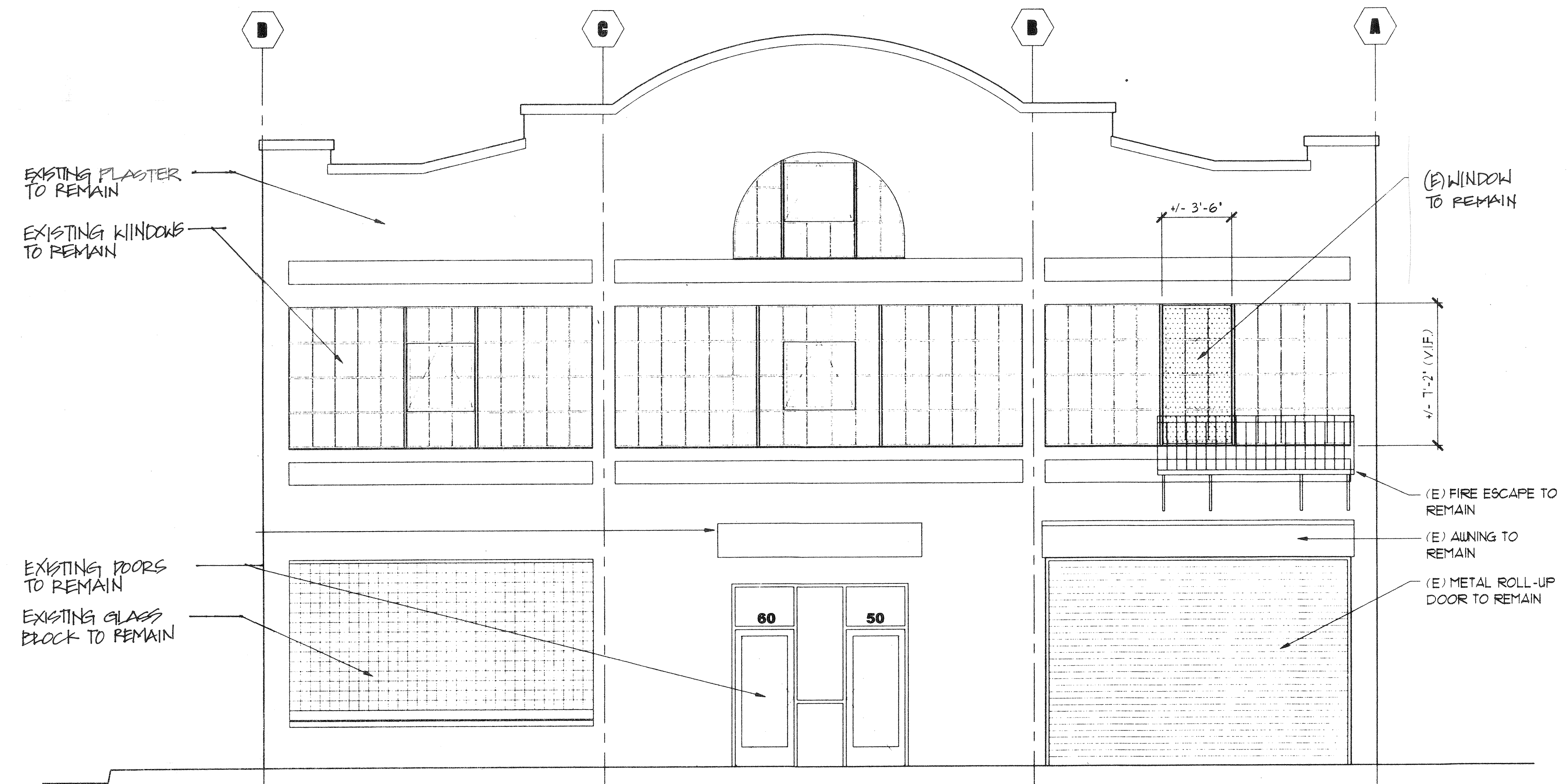
2 SOUTH BUILDING ELEVATION (OTIS STREET) 3.3 1/4" = 1'-0"
