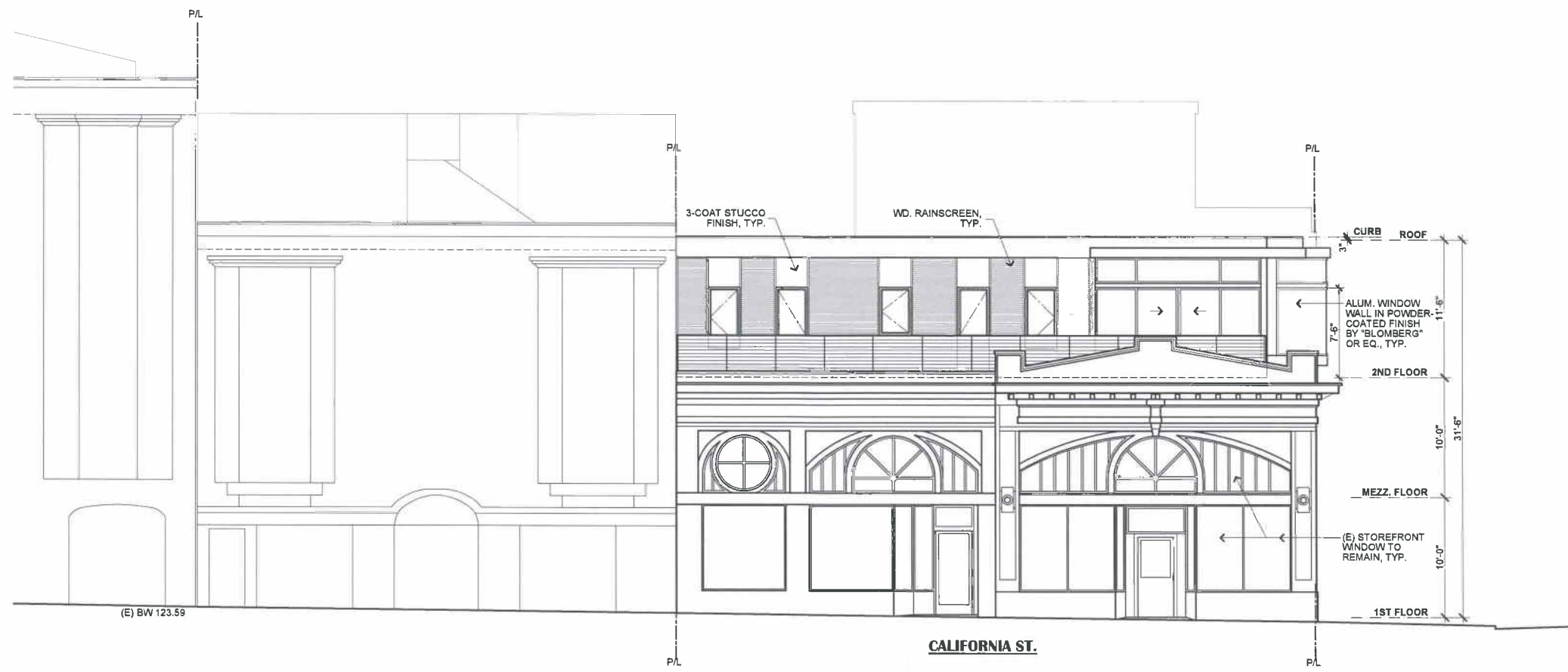
ELEVATION ON CALIFORNIA ST. ALL DIMENSIONS FROM FINISH TO FINISH, U.O.N. SCALE: 3/16"= 1'-0"
