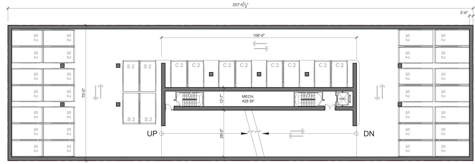
LEVEL B2 40 DOUBLE STACKING CAR-LIFTS 80 MECHANICAL PARKING SPACES TOTAL
