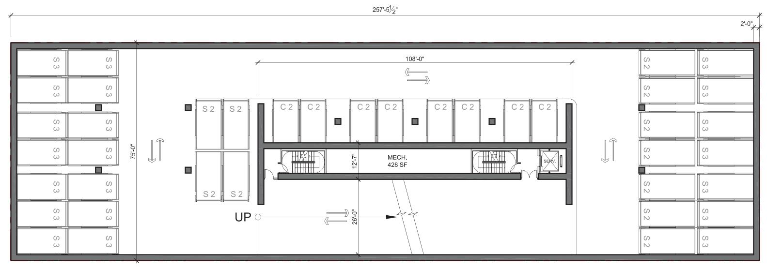
LEVEL B3 - 19 DOUBLE STACKING CAR-LIFTS + 21 TRIPLE STACKING CAR-LIFTS, 101 MECHANICAL PARKING SPACES TOTAL
