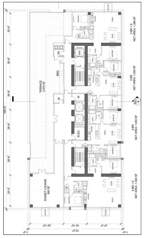
Figure 16 – Proposed Level 31 Floor Plan (Roof Terrace Level)
