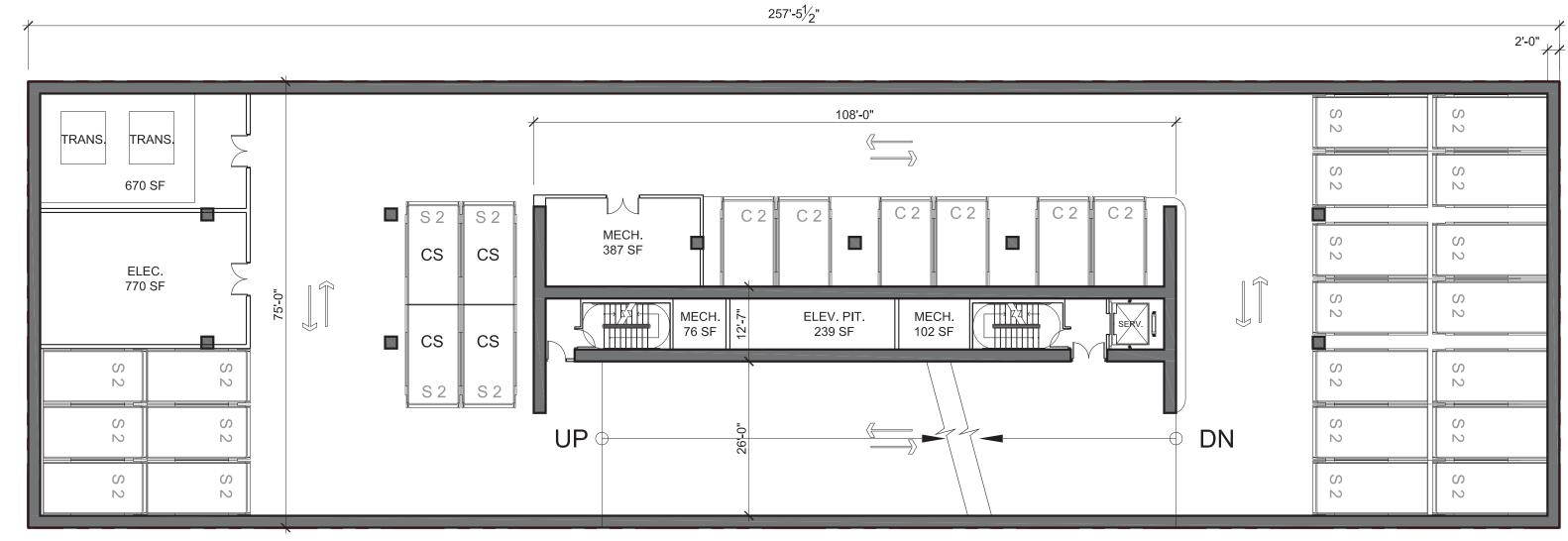
LEVEL B1 30 DOUBLE STACKING CAR-LIFTS, 60 MECHANICAL PARKING SPACES TOTAL
