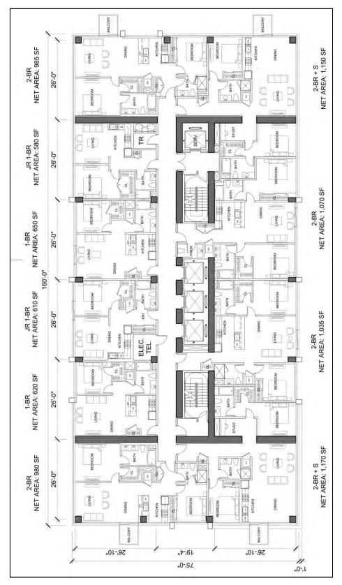
Figure 14 – Proposed Typical Tower Upper Floor Plan (Levels 22 through 28)
