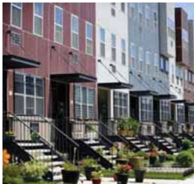
Varying facade colors and materials can decrease the perceived scale of the building
