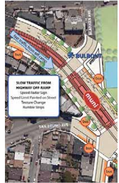
Strategies to slow traffic from the US 101 off-ramp, include rumble strips, speed limit signs, and radar information signs.
