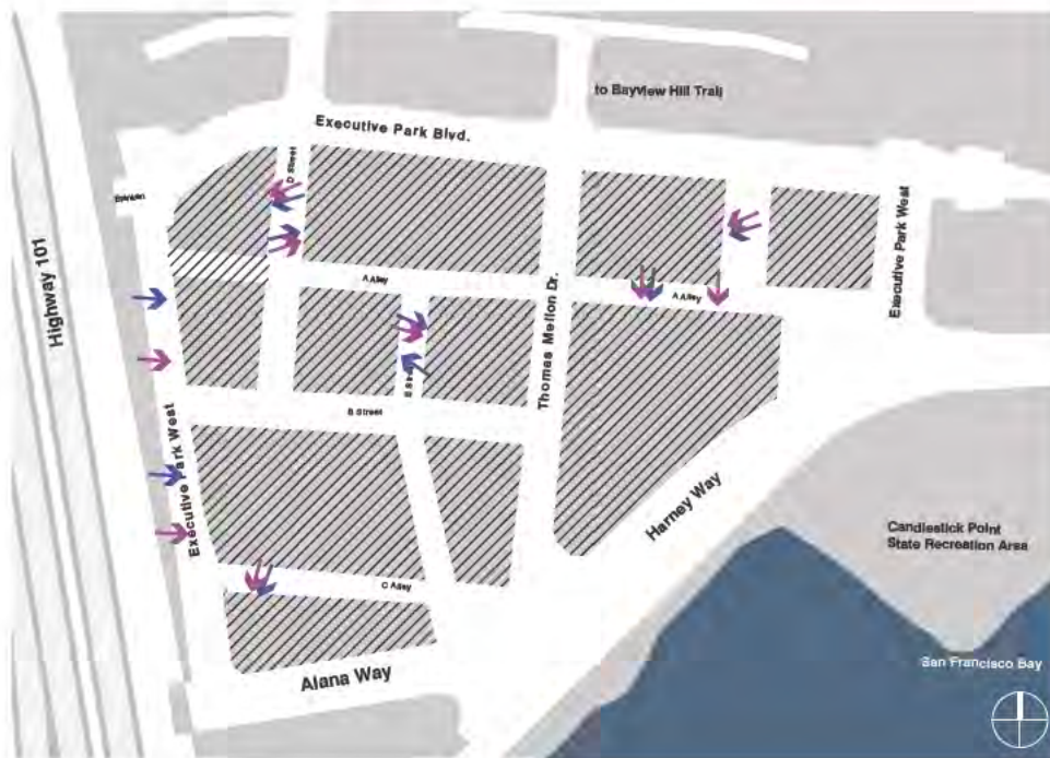
FIGURE D: ALLOWED PARKING AND LOADING ENTRIES. The blue arrows denotes locations of allowed loading entries, the purple denotes locations of allowed parking entry and egress.
