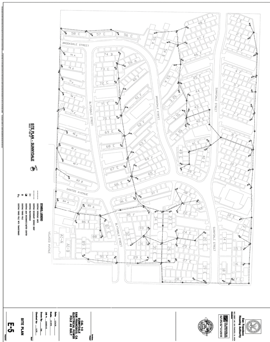
Figure 14.1 – Existing Electrical distribution at Project Site
