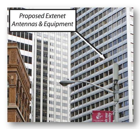
Example of a design that was disapproved by Planning, and is no longer proposed. In this example equipment and cabling below the antenna is not shrouded
