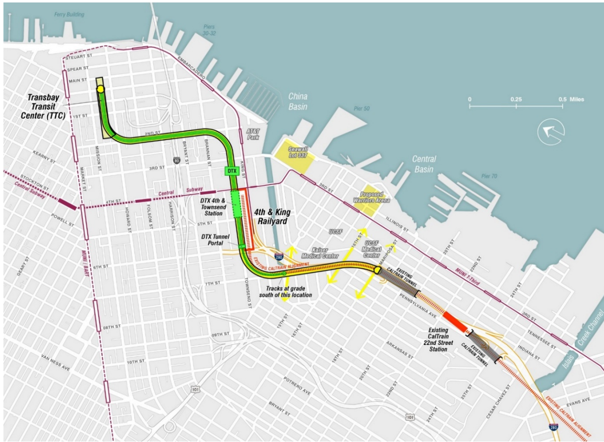
Figure 13: Tunnel Under I-280 Alignment, including planned DTX (in green)
