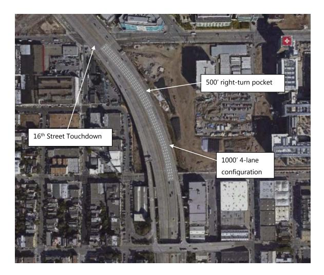
The above mock-up illustrates the extents of the four-lane portion of the exit ramp, along with the 500 foot right-turn pocket.
