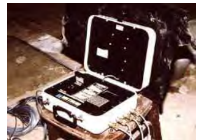
Portable monitors are used to record temperature and humidity conditions in historic buildings during mothballing. Photo: NPS files.
