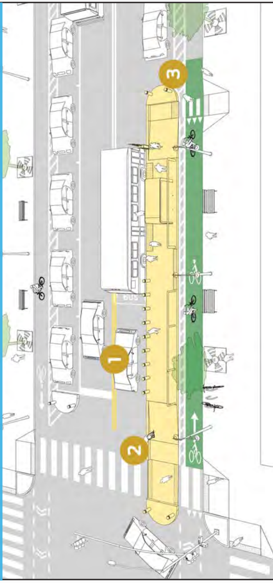
Example: Protected Bike Lane w/Bus Boarding Island
