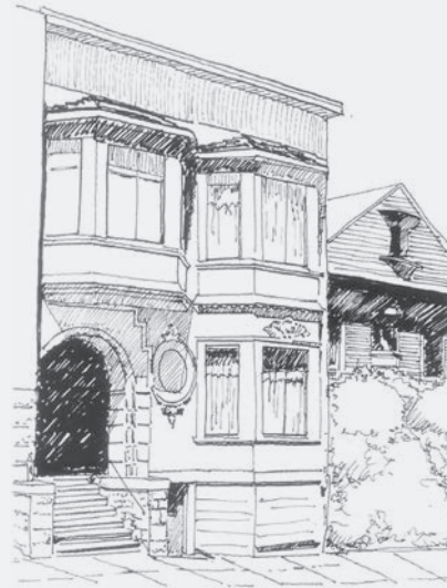
Stairs elevate first floor residential units above pedestrian eye level and provide a transition between public and private space
