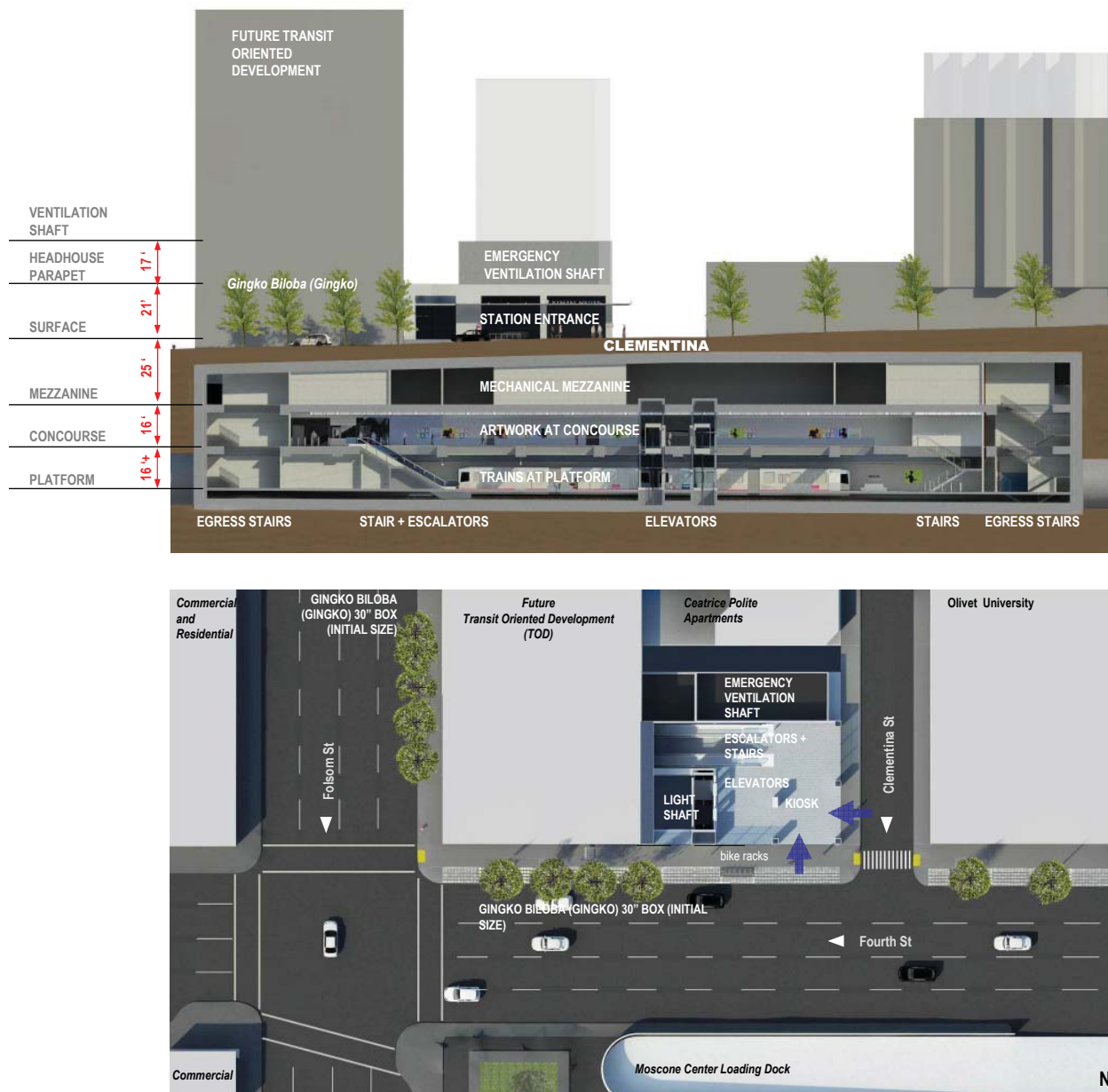
CONCEPTUAL SECTION AND PLAN VIEWS OF MOSCONE STATION (SFMTA)
